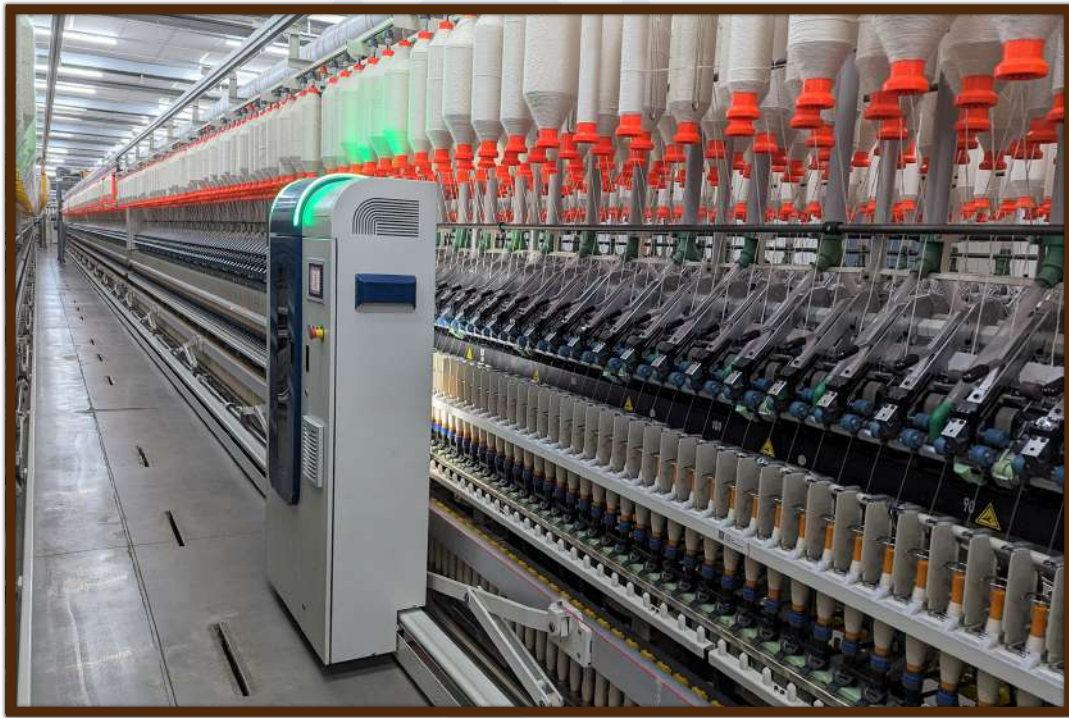
Compact Ring frame LRJ 9/SXL with Ring frame Auto Piecing (RAP)
